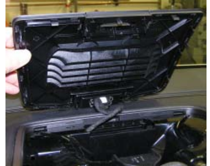
Upper air vent removal
