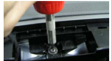
Torx screw to remove shroud
